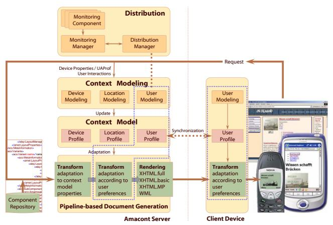
Figure 2: Extended System Architecture Supporting Distribution of Server Tasks (Example: User Modeling)
